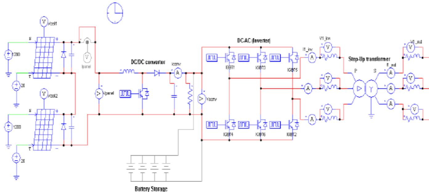
Fig. 5. Grid connected PV system with battery storage modeled on PSIM software
