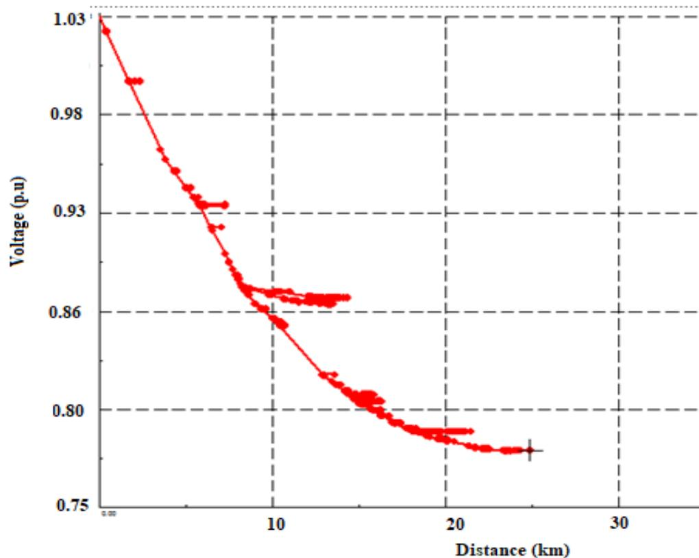
Fig. 10. Voltage profile of feeder X before hybrid system is connected
