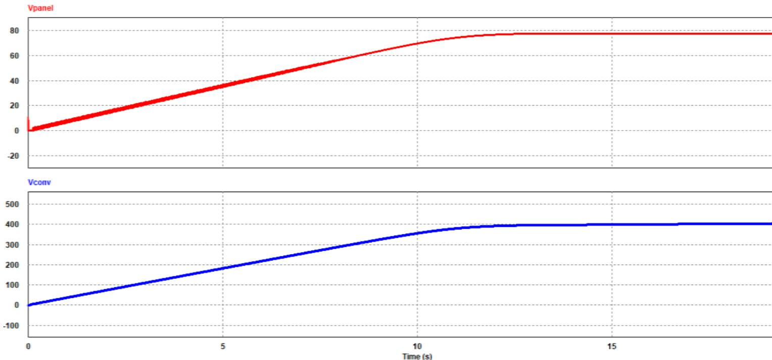
Fig. 6 Voltage from PV panel and converter output
