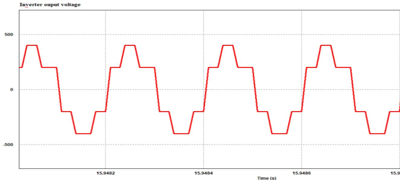
Fig. 7. AC voltage from the inverter
