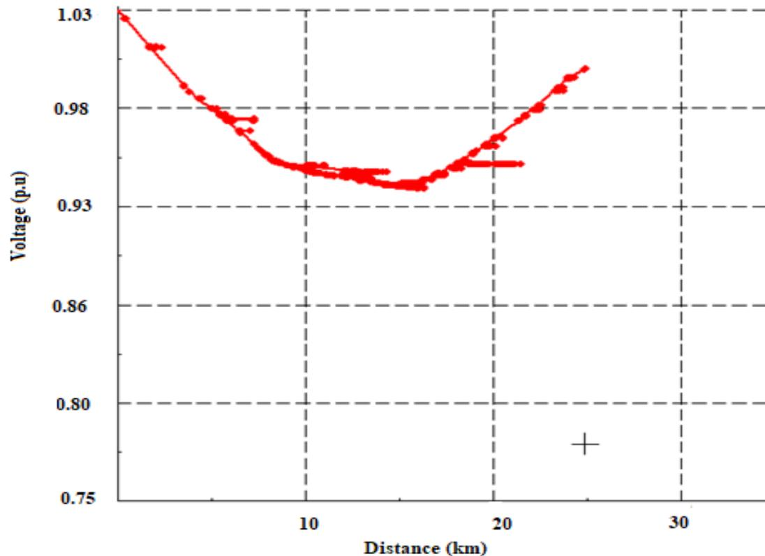
Figure 11. Feeder X voltage profile after hybrid system is connected.
