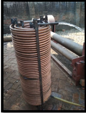
Figure 6. Side view of HE showing the length, spacing of tubes
