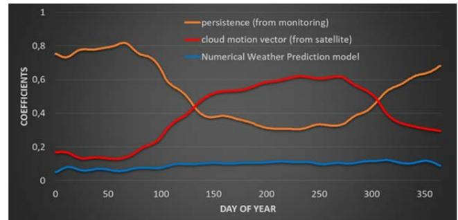
Figure 3. Weighting factors for the 3 input forecasts in dependence of the day in the year. Forecast horizon: 15 minutes.
