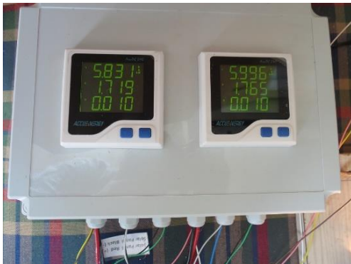
Figure 4. DC Energy meter readings
