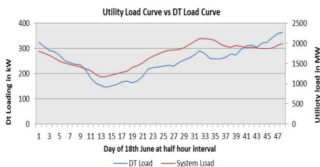
Fig. 1. DT and utility load curve for June 18
