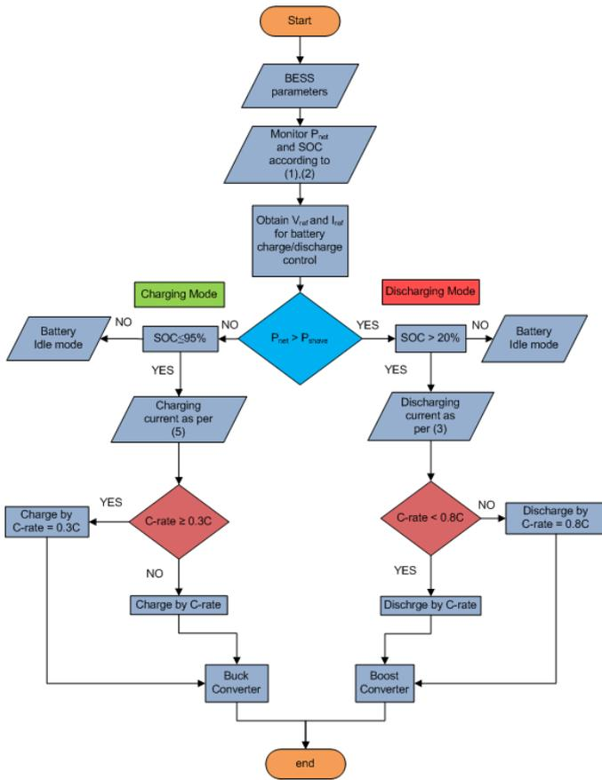
Fig. 3. Flow chart for battery charge/discharge control methodology
