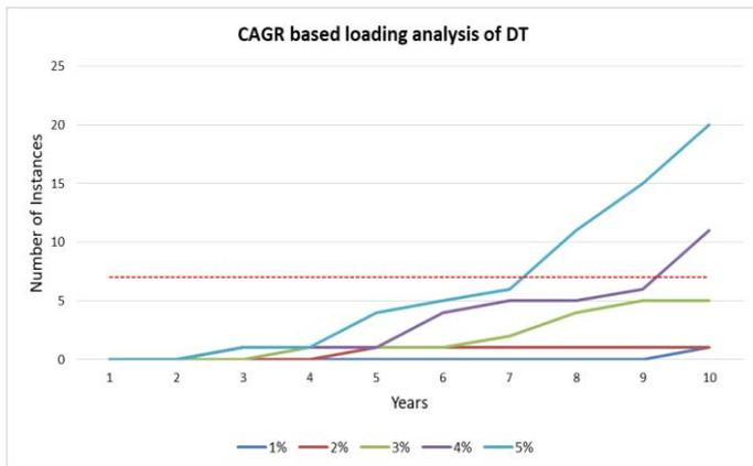
Fig. 6. DT overloading for base-case BESS for different CAGRs over a horizon of 10 years
