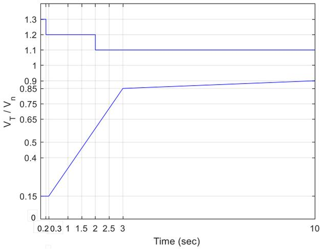
Fig. 1. Lower and upper limit of the voltage-against-time profile of any or all phases at the interconnection point according to the amended CEA Grid Connectivity Standard [12].
