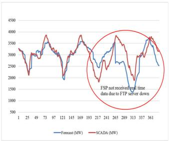
From the above, it is emerged that SLDC could not rely on decentralized forecast received from various pooling stations as well as centralized forecast received from FSP. Therefore, it is necessary that FSP should develop such robust model that could not depend on loss of real time generation data or weather data. Also, the redundant communication links / equipments / hardware are required be provided to get real time data to SLDC and further extending to FSPs.
