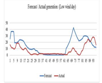
It is observed that there is vast difference between decentralized forecast and actual provided by CA. In high wind scenario, the actual wind generation remains on higher side whereas it remains less in low wind scenario.
