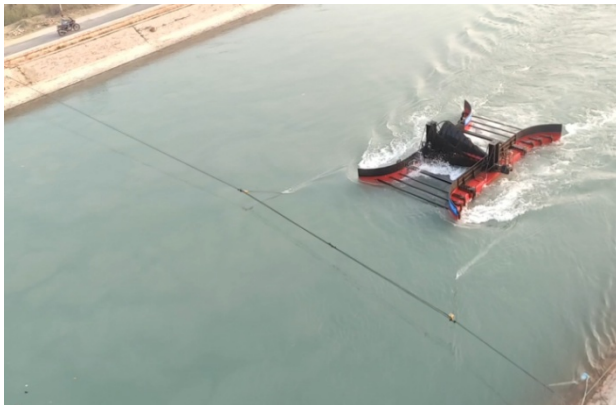
Figure 8, Area View of VARUN-III Turbine Module installed in floating condition.
