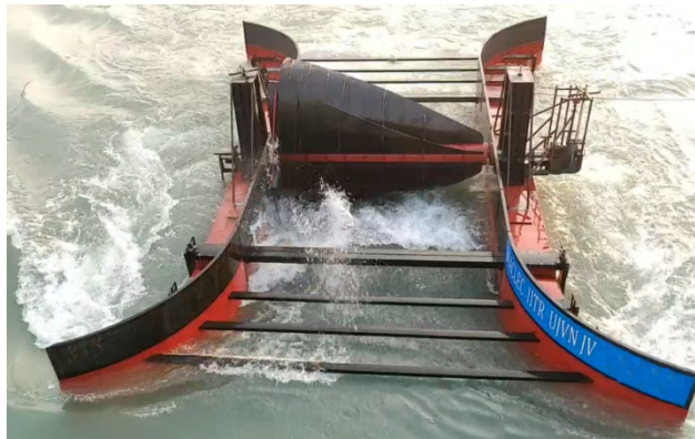
Figure 3, 5 kW Prototype of the Proposed technology installed at upstream of Upper Ganges Canal, Uttarakhand.
