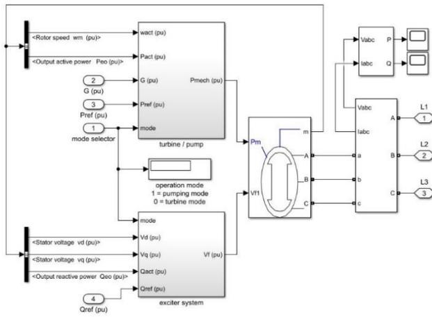
Figure 7. Pumped-storage power plant model
