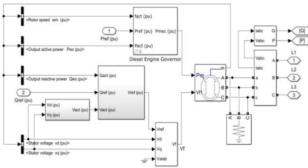
Figure 11. Diesel generator model
