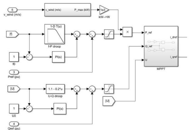
Figure 10. PQ control mode of photovoltaic and wind turbines
