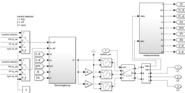
Figure 8. Selection of reference values for  $i_d$  and  $i_q$  for PQ mode
