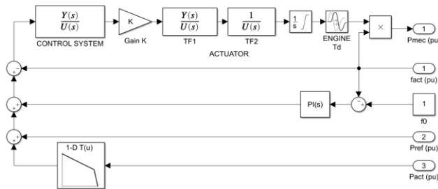
Figure 12. Diesel generator model
