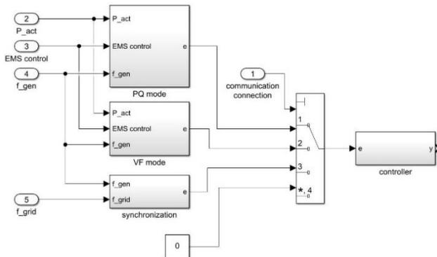
Figure 2. Controller structure of renewable energies
