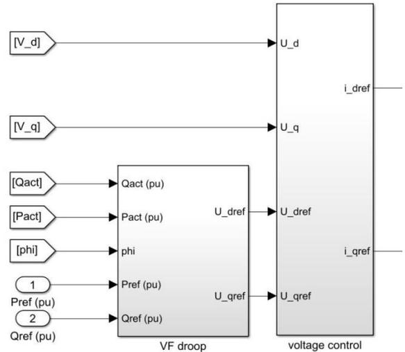
Figure 9. Selection of reference values for  $i_d$  and  $i_q$  for VF mode
