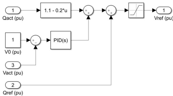
Figure 13. Determination of reference voltage  $V_{ref}$
