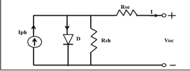
Figure 1. Equivalent circuit of a PV cell
