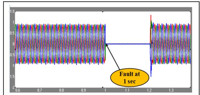
Figure 12. Voltage at PCC during three phase to ground fault
