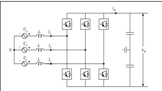
Figure 4. Two level voltage source converter
