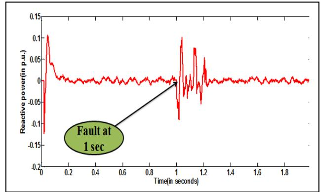
Figure 19. Reactive power during fault at 1-1.2second
