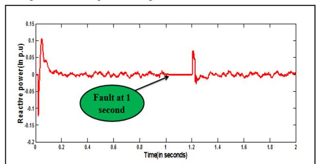
Figure 15. Reactive power during fault at 1-1.2second
