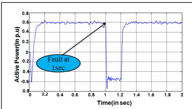
Figure 18. Active power during fault at 1-1.2seconds
