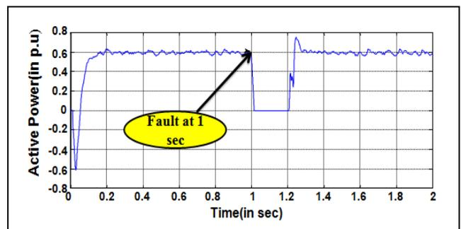
Figure 14. Active power during fault at 1-1.2second
