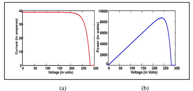
Figure 6. Maximum Power delivered by PV system (b) Current in PV system
