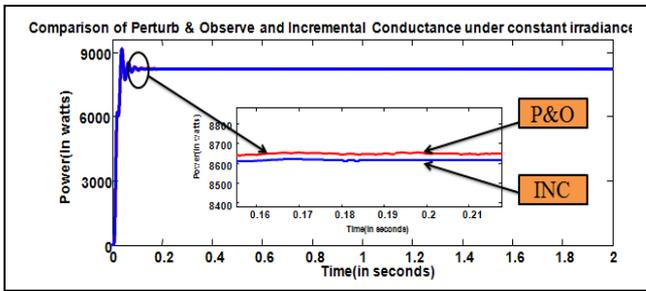
Figure 7. Comparison of P&O and INC under constant irradiance
