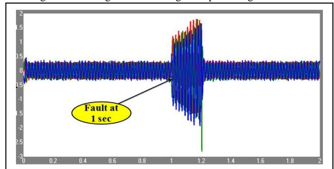
Figure 13. Current at PCC during three phase to ground fault
