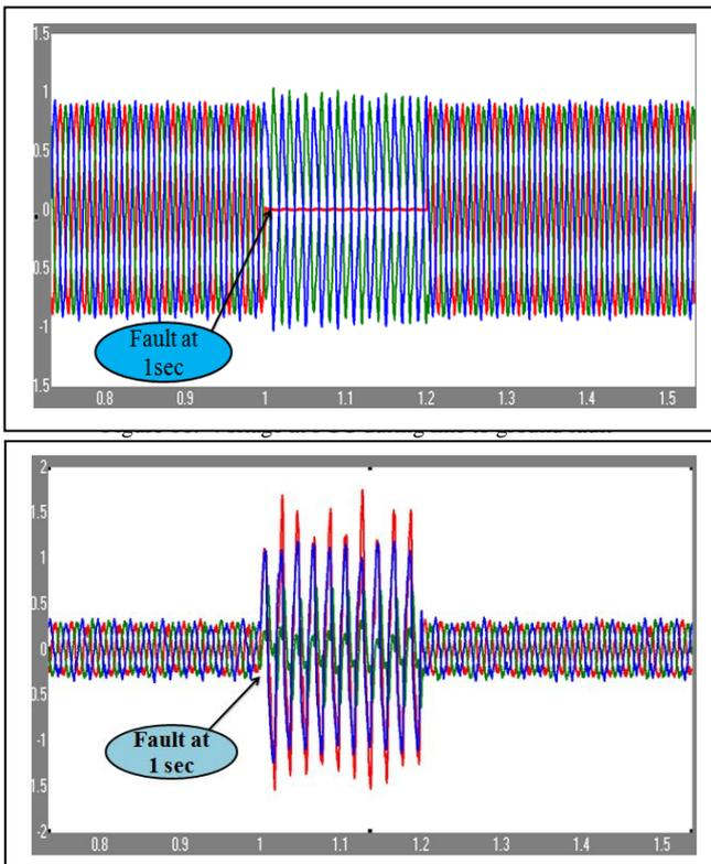
Figure 17. Current at PCC during line to ground fault
