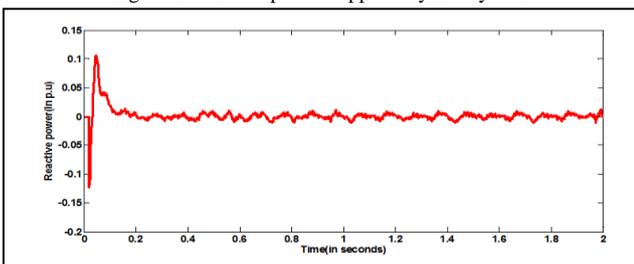
Figure 11. Reactive power supplied by the PV system
