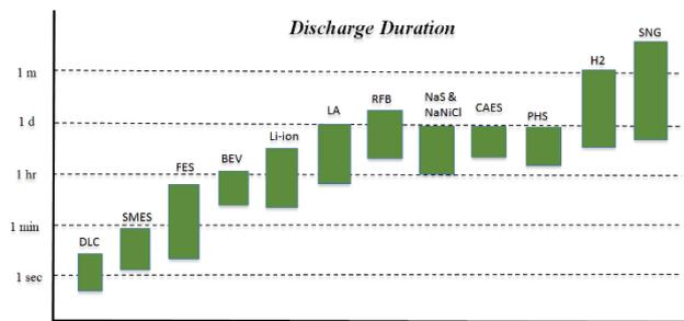
Figure 3: Discharge duration of different types of storage technologies
