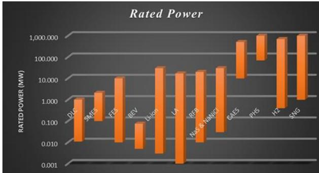
Figure 2: Rated power of different storage technologies
