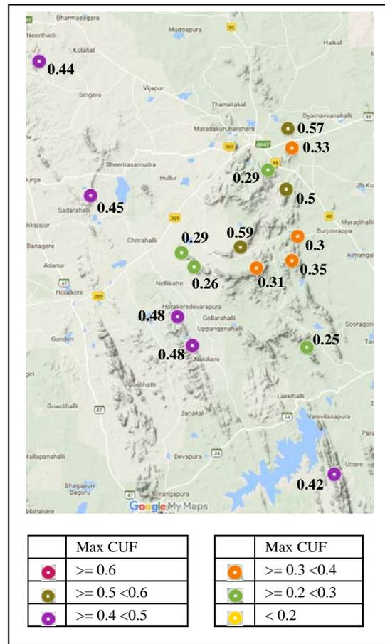
Figure 5. Maximum Capacity Utilization Factor for various wind power plants in Chitradurga Region during Monsoon of 2015 and 2016
