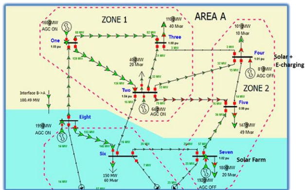
Figure 4. Multi-Bus Power network
