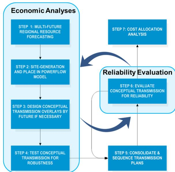
Figure 4. MISO’s value based planning process
