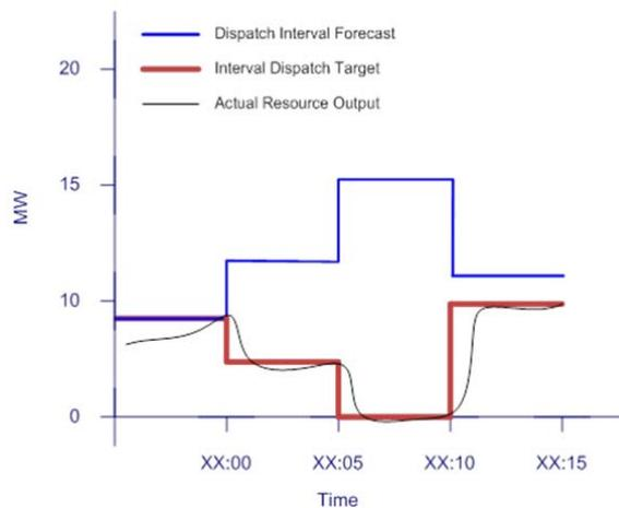
Figure 11. DIR following dispatch in a constrained system
