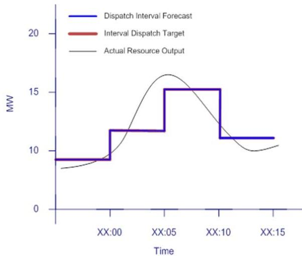
Figure 10. DIR following dispatch in an unconstrained system
