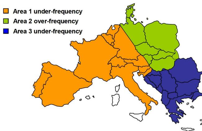
Fig. 4. Schematic map of UCTE area split into three areas [13]
