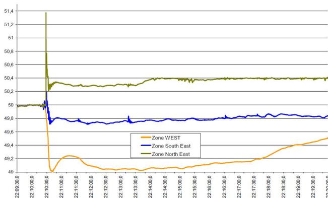
Fig. 5. Frequency recordings after the split [13]
