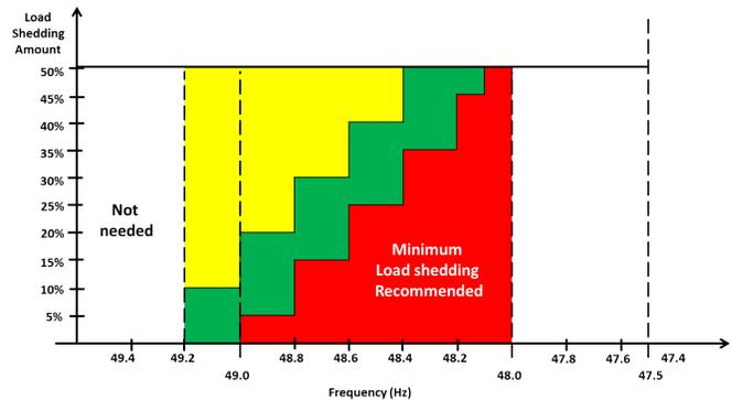
Fig. 10. ENTSO-E Recommendation for UFLS [21]
