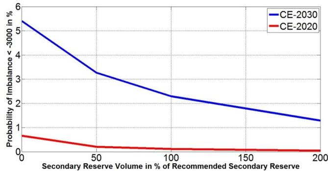
Fig. 6. Probability of power imbalance exceeding 3000 MW for CE for different volume of secondary reserve
