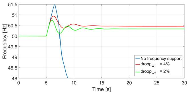
Fig. 9. Frequency with 40% Wind Power Penetration in Area 1 in PEGASE network
