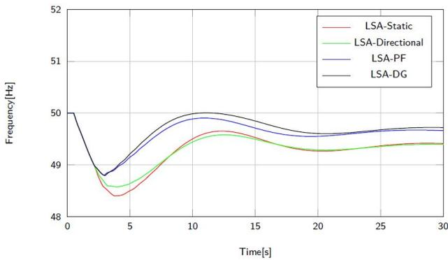
Fig. 11. Frequency responses for different load shedding schemes
