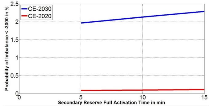
Fig. 7. Probability of power imbalance exceeding 3000 MW for CE for different activation time of secondary reserve
