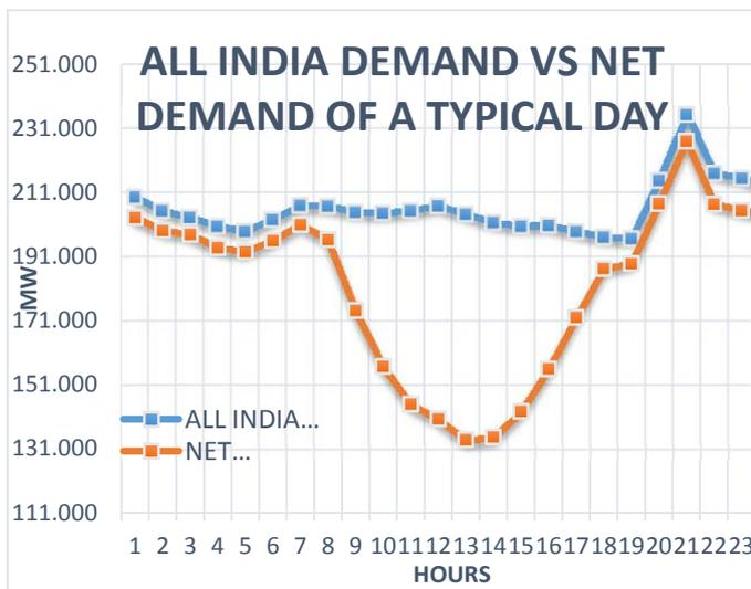
To cater to the Huge peaking requirement, gas power plants and hydro power plants especially pumped storage type hydro plants will be required. Other storage technologies like large capacity batteries which are in nascent stages of development can also contribute in meeting the peaks. Economic viability of all such balancing technologies will need to be assessed so that the electricity is within the reach of every consumer at affordable rates.
