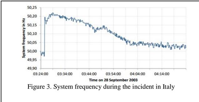
Figure 3. System frequency during the incident in Italy
