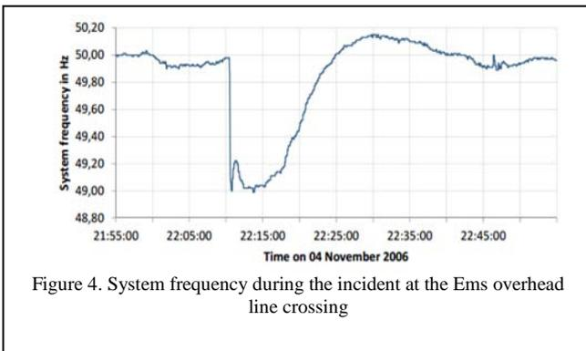
Figure 4. System frequency during the incident at the Ems overhead line crossing
