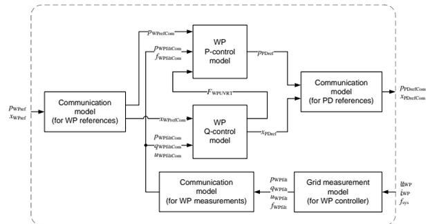
Figure 4. General modular structure of the wind power plant control and communication block.
