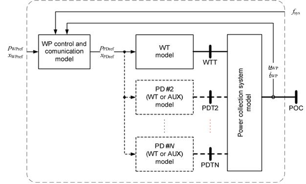
Figure 3. General modular structure of the wind power plant model.
