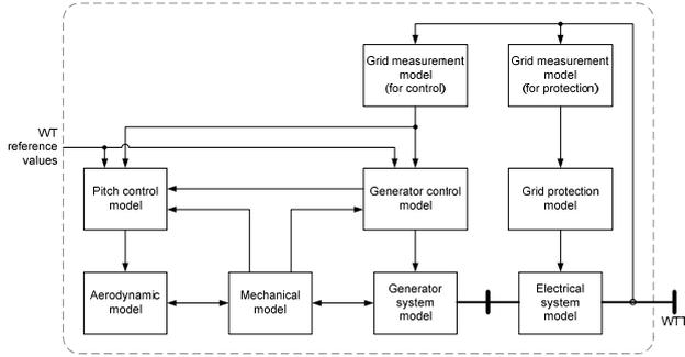
Figure 2. General modular structure of 2<sup>nd</sup> edition wind turbine models.
