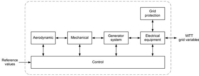
Figure 1. General modular structure of 1<sup>st</sup> edition wind turbine models [7].
