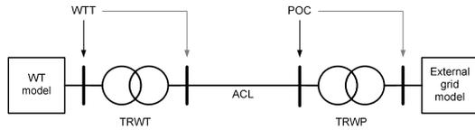
Figure 5. Single line diagram for the basic wind power plant model
