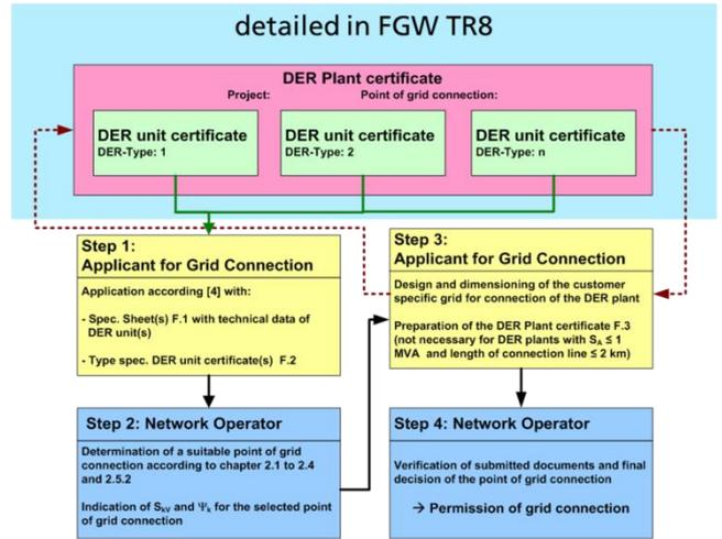
Figure 2. Approval procedure acc. to German MV-Grid Code [5]
