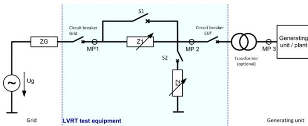
Figure 6. UVRT test equipm. acc. to IEC 61400-21 [16], FGW TR3 [7]
