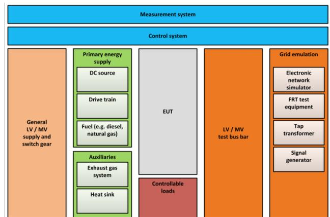
Figure 7. Testing laboratory building blocks and conceptual arrangement
